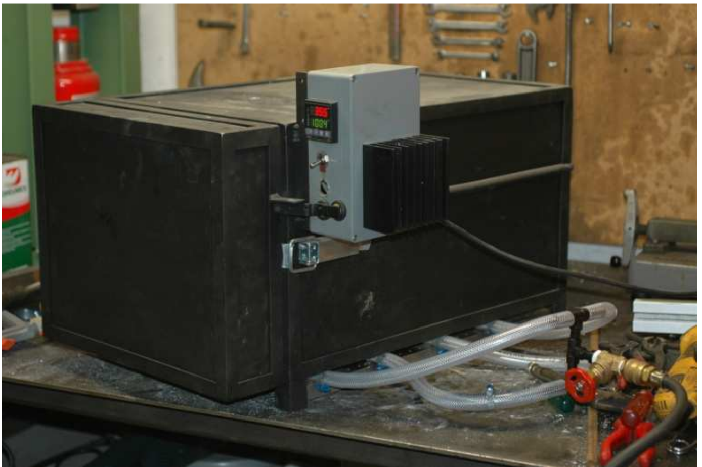
Fig. 8. The heat treating oven with air tubing
