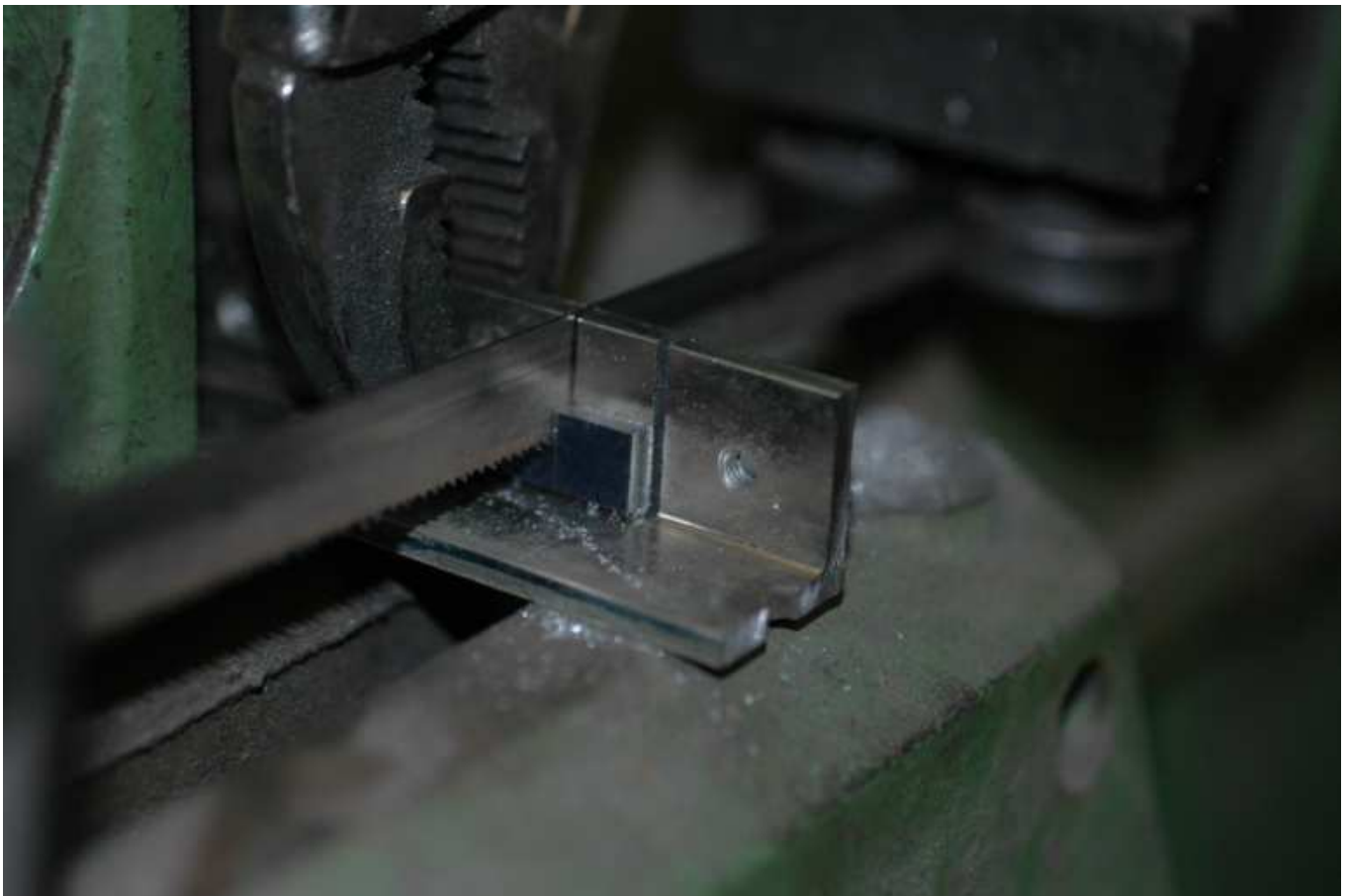
Fig. 4. The samples being cut on a bandsaw
