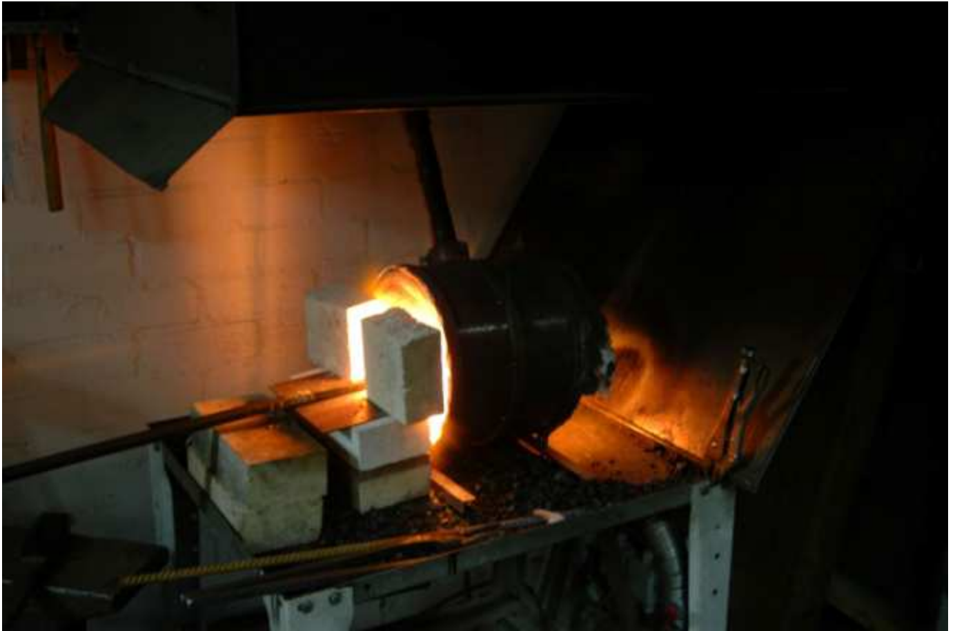
Fig. 3. The propane-butane fired forge at welding temperature
