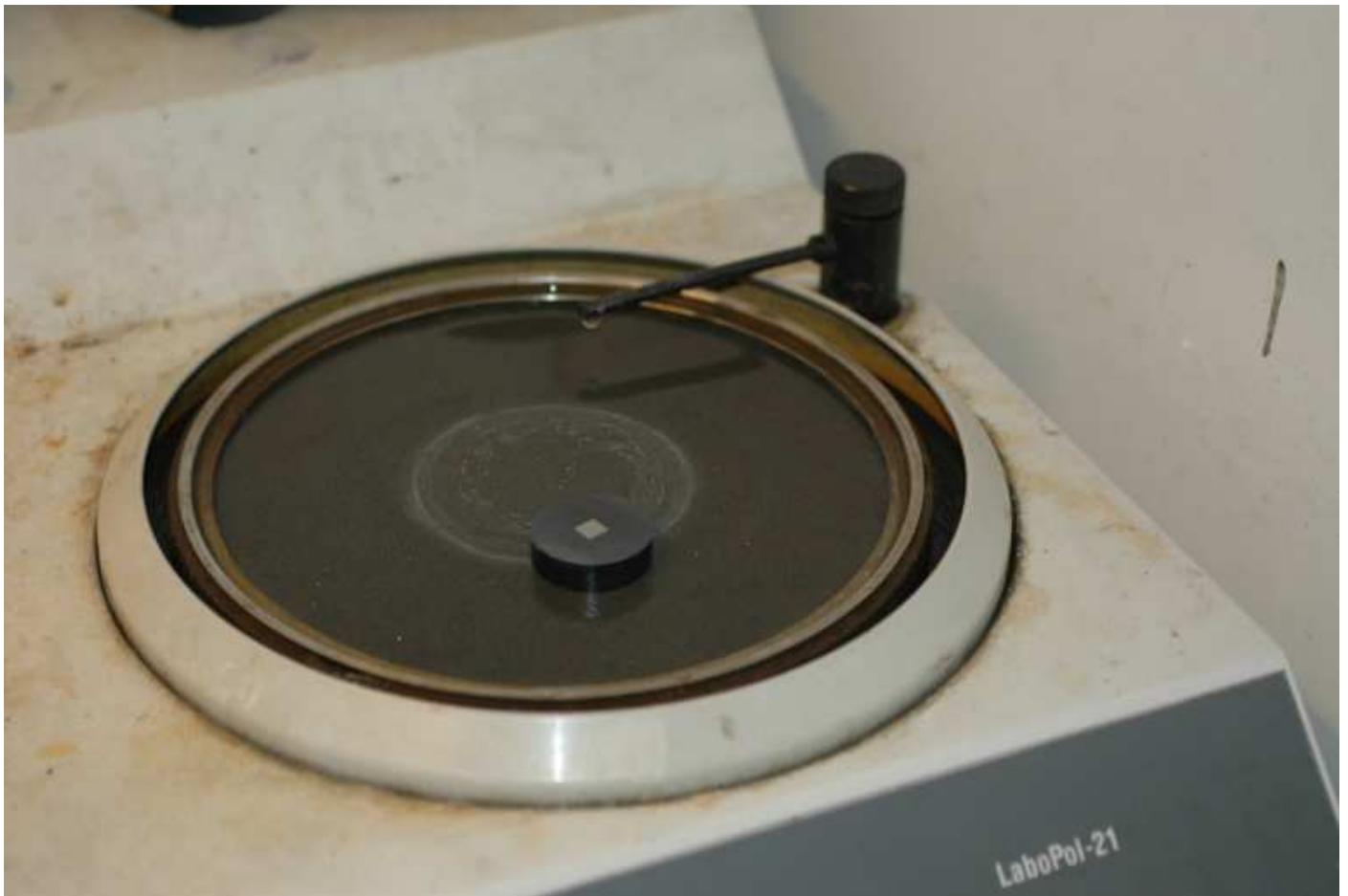
Fig. 11. An embedded sample on a grinding disc.
